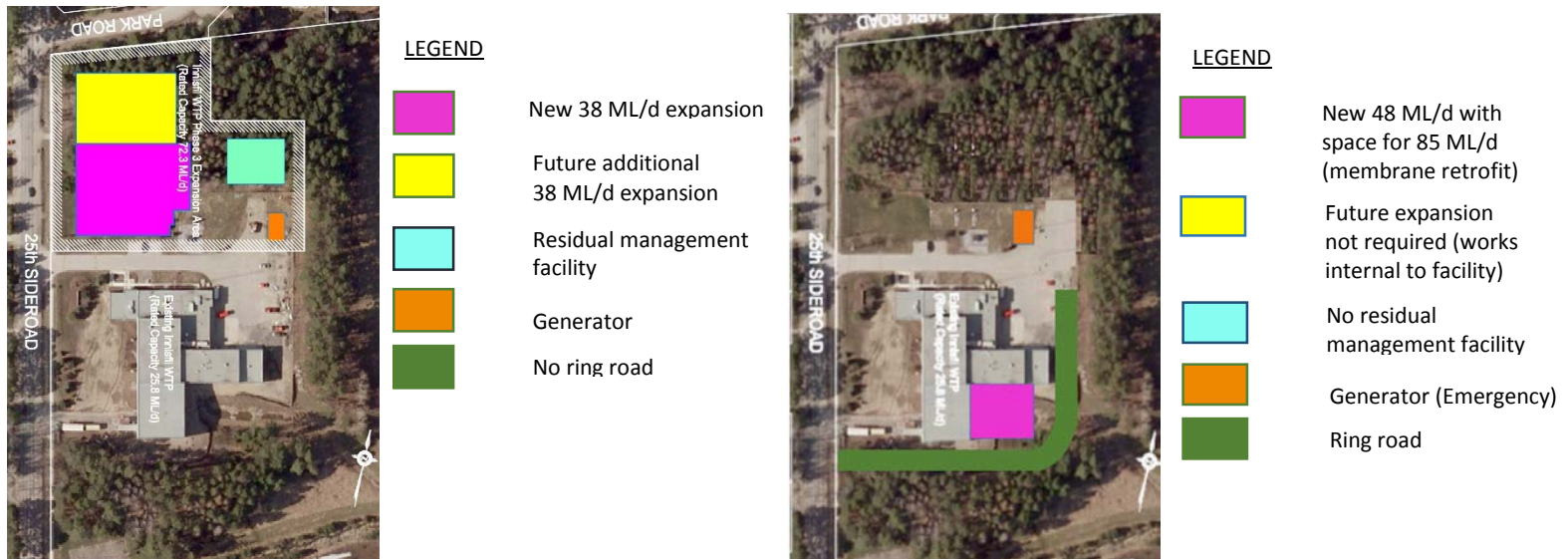
Figure 7.4.1: WTP Expansion Comparison
